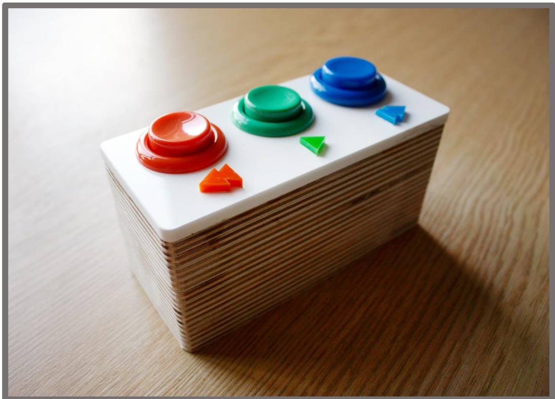
Figure 29 - PowerPoint control console
