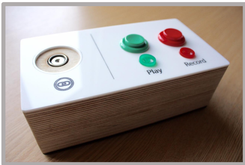
Figure 19 – Tag reader with 1-wire tag reader on left hand side
