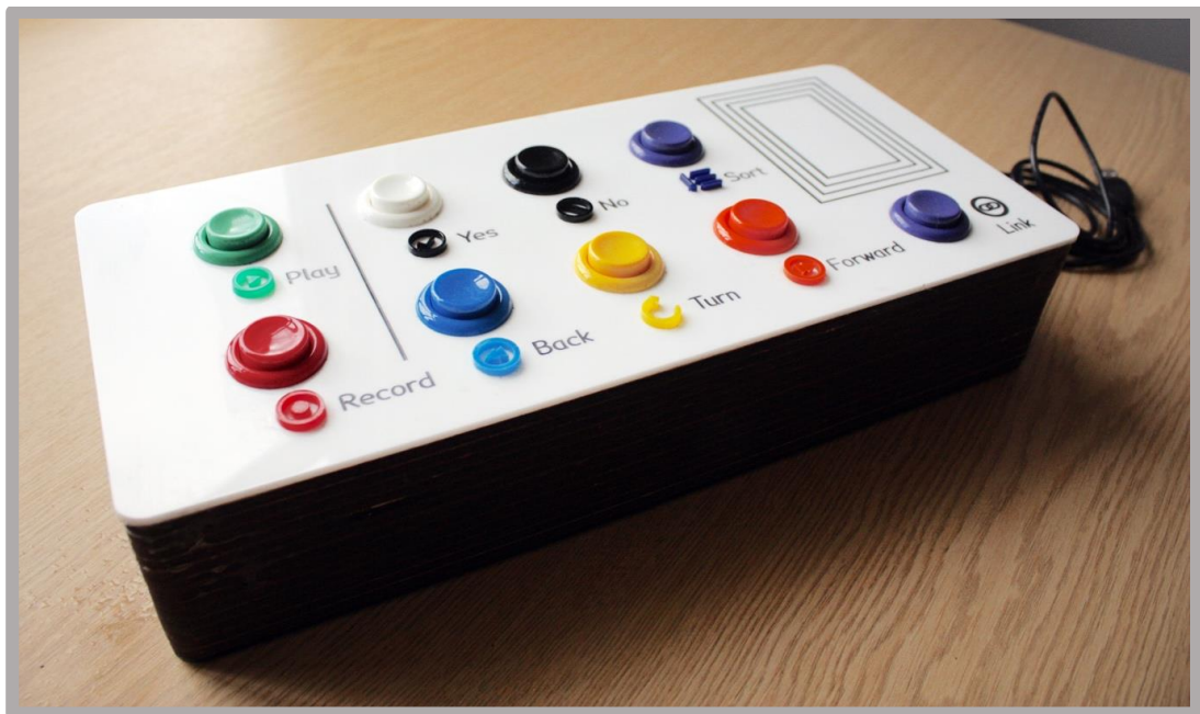
Figure 23 - Console 2 with built in RFID reader and 'sorting button'.
