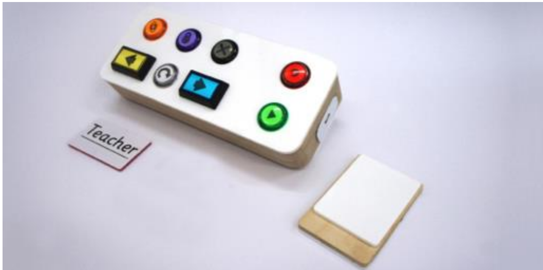
Figure 11 - Photo-sorting console with RFID card & reader
