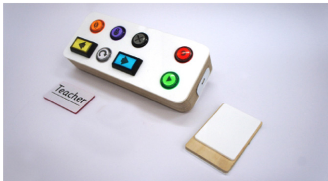
Fig. 4. Photo-sorting console with RFID card & reader.
